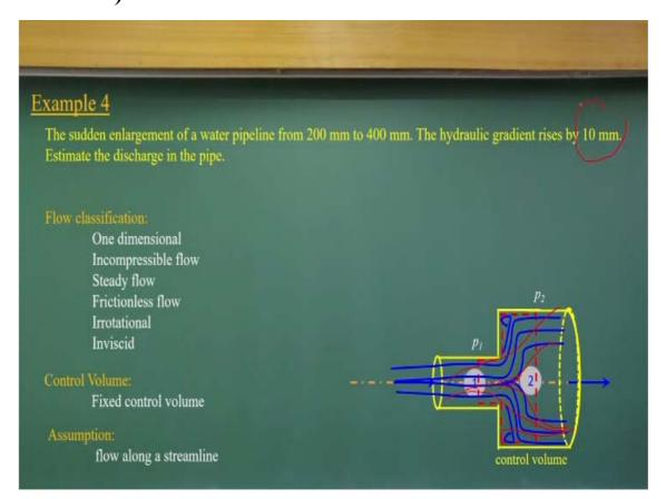
Another problems, we are very interesting problem, here there is sudden enlargement of pipeline from 200 millimeter to 400 millimeters. The hydraulic gradient raises by 10 mm okay. It is just given, their hydraulic gradient lines has increased by 10 mm. Then, we can estimate what will be the discharge in the pipe. So, again we will apply same mass conservation equation and the energy conservation equations around the streamlines. You can see that mostly the streamlines will have a divergent.
