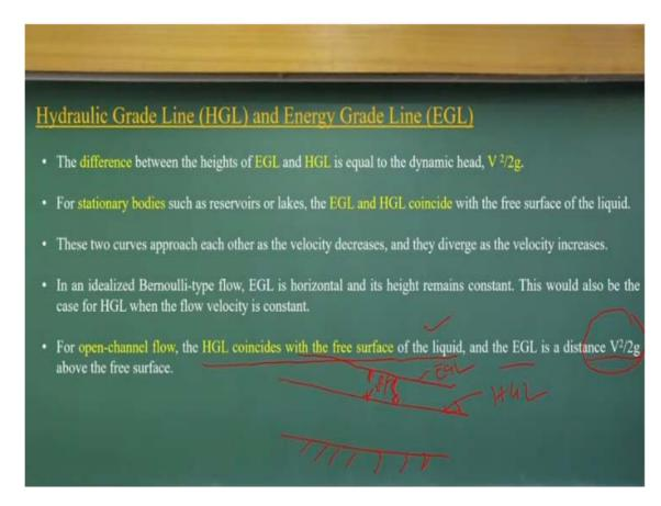
And okay, we are not discussing about open channel flow heads, but in case of open channel flow, the hydraulic gradient lines coincides with the free surface of the liquid okay. Because there is no pressure head. So, whatever the water surface free surface, that what will be hydraulic gradient line and the energy gradient lines will have a included the velocity head above the free surface. That means, if you consider a open channel flow, this is the free surface.
