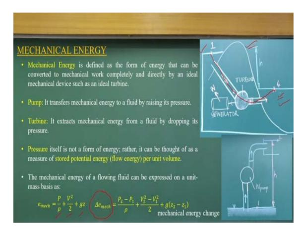
Now, let us consider is the problems when we generally use as a engineer having a pump and turbine systems. As you know it, the pump is transfer from mechanical energy to fluid by rising pressures, okay. Transfer the mechanical energy to a fluid. So, fluid gains the energy because of the pumping systems by rising its pressures, that is the. Similar way, the turbine does opposite things, that it takes out or extract the mechanical energy from the fluid by dropping it pressure.
